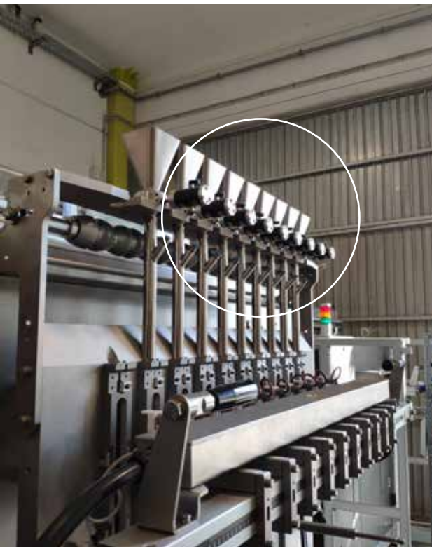
K (linear pneumatic vibrator) - Hopper emptying
